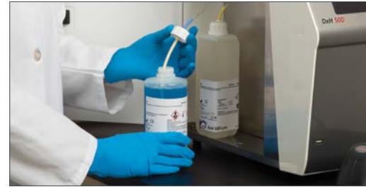
Each reagent can be changed out individually in less than 2 minutes.
